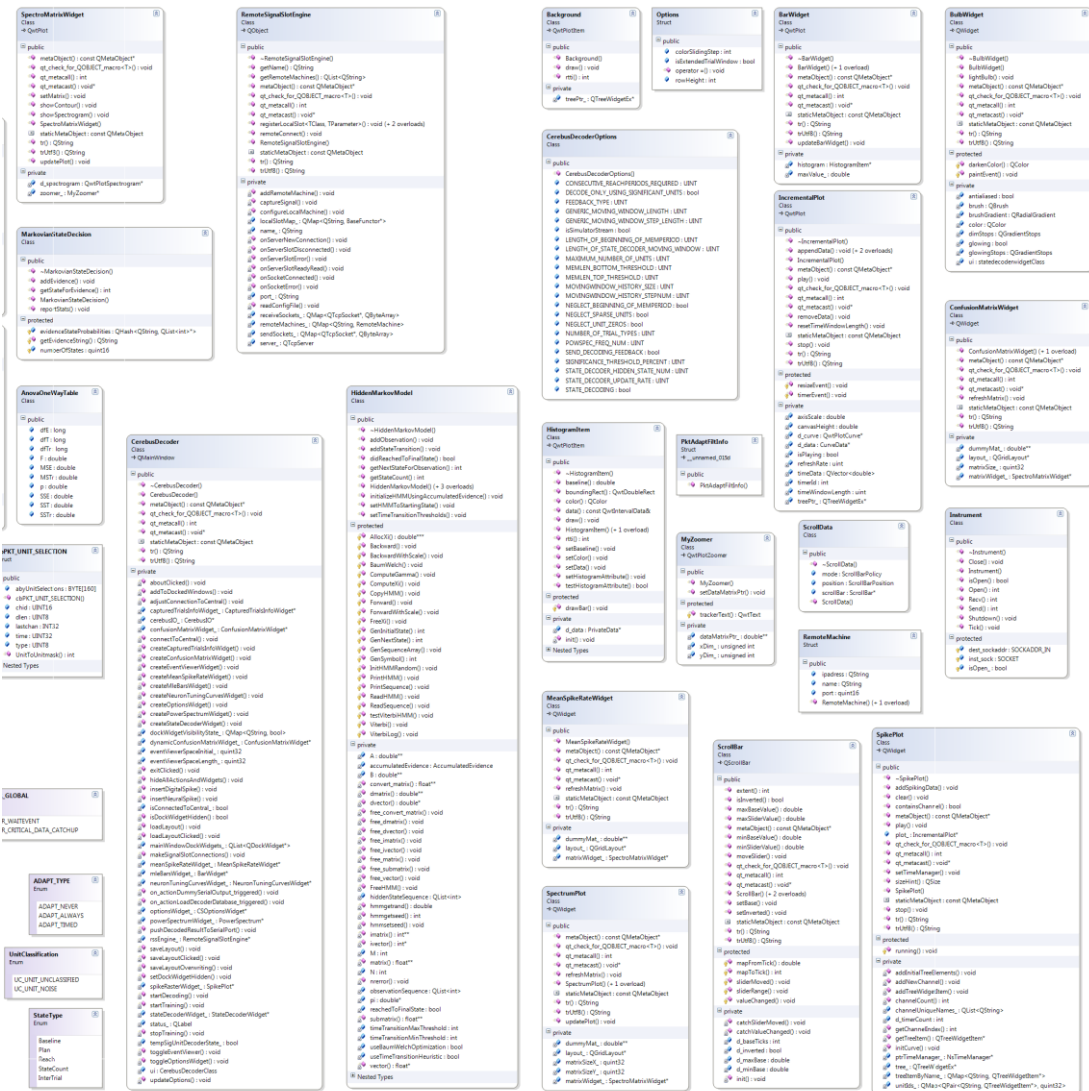
Figure Appendix-B.4: Expanded class diagram for Decoder Software, part 1. The attribute and method names for user interface and some utility classes and data structures of Decoder software.
