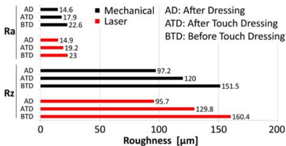
Fig. 9. Comparison of Ra and Rz-roughness values before and after touch dressing and after the SiC dressing process.
