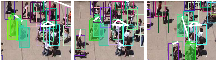
Figure 7.10: Tracker failure detection. Sometimes, the initialization or the tracker itself lead to a wrong estimate. The leftmost figure shows such a case, where for the two subjects with ID 28 and 35, there is another pair of wrong estimates, namely 50 and 46. The tracks of interest are represented with a shaded bounding box. The tracker finds out that the estimates are wrong in the following frames. This happens because the wrong tracks violate the avoidance behaviors, since they overlap with other tracks and lack of a strong observation support. We show frames, from left to right 1175, 1200 and 1250.
