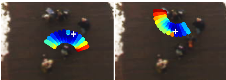
Figure 4.1: While walking among other people, several factors influence short-term path planning. Smoothness of motion, intended destination, and interactions with others limit one’s choice of direction and speed. In the example (same scene, two pedestrians’ perspectives), blue indicates good choices for velocity, red signals “no-go”s. The white cross shows the actually chosen velocity.
