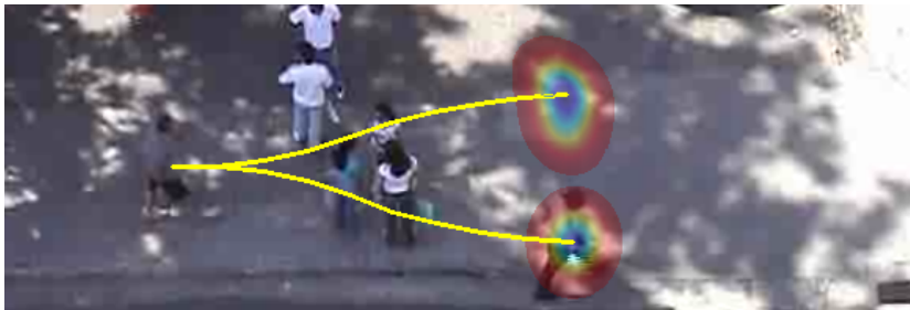
Figure 5.1: When moving through a scene, a person takes a variety of factors into account, such as steering clear of other people. In many cases, the prediction of the motion cannot be well described by a deterministic algorithm: in the above example the pedestrian on the left hand side could either evade the group by going on its left or right side, as indicated by the yellow lines. We therefore propose a stochastic extension of LTA that can deal with the uncertain future motion of a pedestrian.
