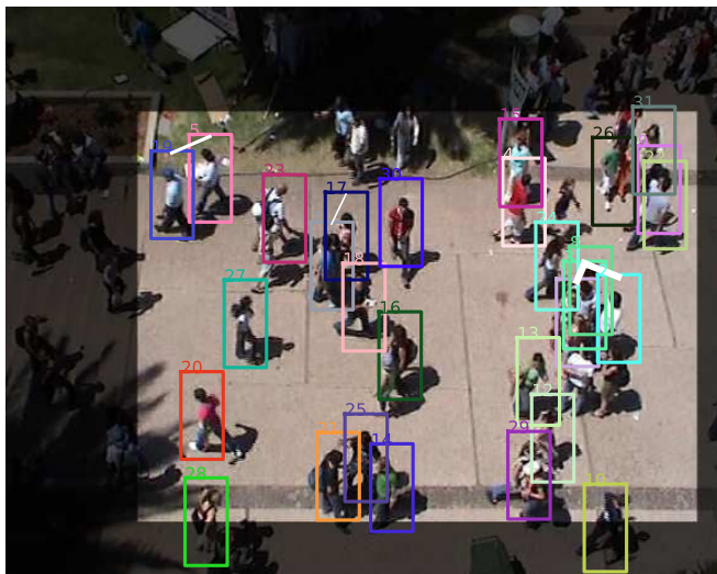
Figure 7.5: A result frame from the Students sequence. The white line connecting the bounding boxes shows the group relationship estimate. The thicker the line, the stronger is the estimate that the two connected subjects belong to the same group.
