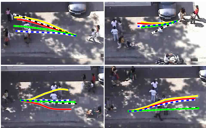
Figure 4.5: Example extrapolations: the model smoothly avoids the standing crowd (top left, yellow=groundtruth), sometimes however suggests meaningful, but wrong paths (bottom left). Using only goal-directed prediction is effective in some cases (top right) but in general better prediction is obtained by taking into account interaction among pedestrians (bottom right).
