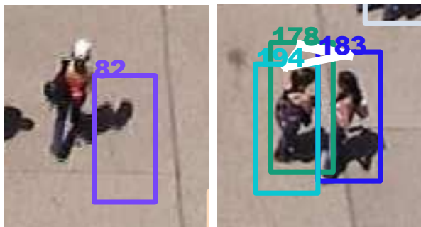
Figure 7.9: Tracker errors. Some of the tracker errors are caused by a wrong initialization. In the left figure, the shadow is detected instead of the person. Furthermore, the shadow moves indeed like a human, and this makes it harder for the inference to infer that there is a failure. The right figure shows another mistake. This time is the bag that is being recognized as a person and is also being assigned the same group as the other two subjects.
