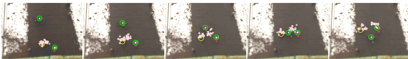
Figure 5.4: Particle filter experiment: when simulating a person (yellow circle) given the other people (green circles) using a particle filter embodiment of the model, multiple modes (red particles) form naturally. While both options of steering clear of the oncoming persons are found, such a solution is computationally prohibitive (see text).
