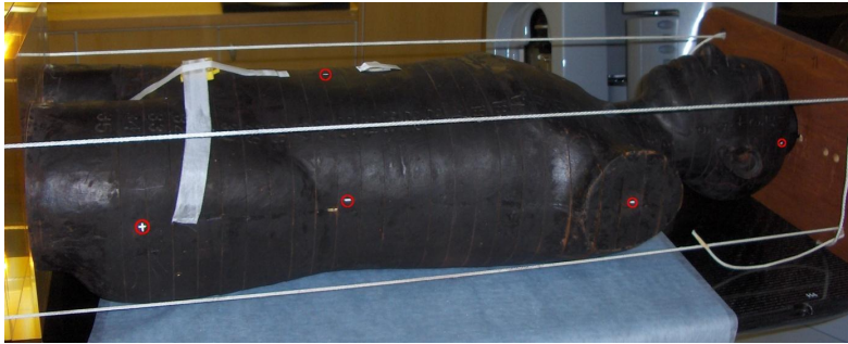
Figure 5.12: Markers for the laser system on the Alderson phantom.
