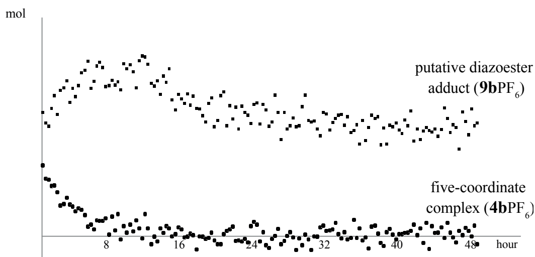
Figure 2.10 Reaction profile of a catalytic run performed with 4bPF 6 at 0 °C as monitored by 31 P NMR spectroscopy (283 MHz, CD 2 Cl 2 ) during 48 h. The 31 P NMR spectra were recorded every 10 min and the integration of the signals is plotted against time.
