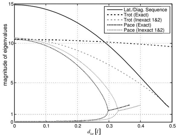
**Fig. 7** Magnitude of the roll-mode for the different 3D gaits. This mode is unstable for all gaits and the possible range of lateral leg spacing. Gaits that show more pronounced energy losses due to lateral motion (such as the pace) have a ‘less unstable’ roll-mode, in the sense that disturbances grow slower.
