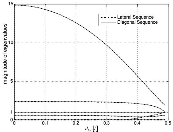
**Fig. 4** Eigenvalue magnitudes for varying width of the main body (lateral leg spacing) for the lateral and diagonal single foot sequences are absolutely identical. The two gaits are equivalent with respect to stability.
