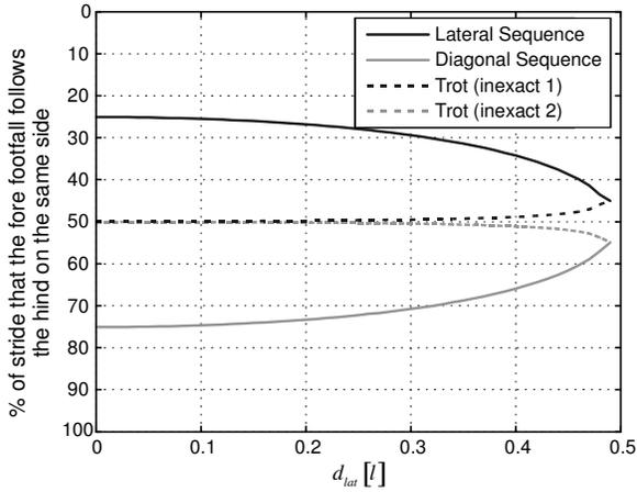
**Fig. 5** Phase shift (in percent of a total stride) between the back and front legs on the same side of the quadrupedal model as a function of lateral leg spacing. For increasing lateral leg spacing, the four-beat gaits (in lateral and diagonal sequence) converge towards a trotting gait, while the inexact trots diverge towards more pronounced four-beat gaits. At the critical leg spacing of  $0.49l$  four-beat and inexact trots become identical and cease to exist for even wider leg spacing.
