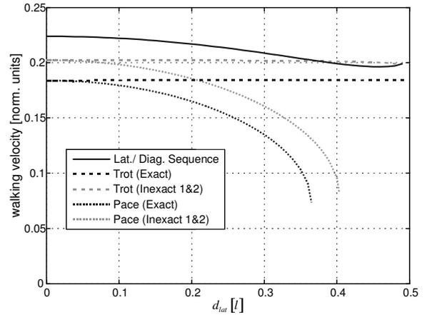
**Fig. 6** Walking velocity (in normalized units  $\sqrt{gl}$ ) for the different 3D gaits as a function of lateral leg spacing. No difference in walking speed exists between the lateral and diagonal single foot sequences as well as between the different kinds of inexact paces and trots. While the trots are nearly unaffected by the leg spacing, the lateral rocking motion in the paces dissipates energy slowing down the forward motion.
