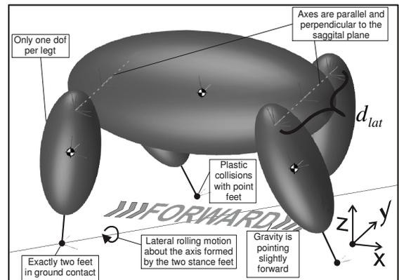
**Fig. 3:** Model of a three dimensional passive dynamic quadruped. While the internal dynamics of the model are planar (all legs swing in parallel planes), it can rotate freely about the axis defined by the stance feet on the ground, which adds an additional degree of freedom in comparison to the planar model described in [9]
