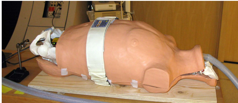
Figure A.1.: Anthropomorphic respiratory phantom. Motion is induced by inflation and deflation of the lung cavities by way of the pipe visible at the cranial end of the phantom. The actual extent of the motion is measured in the SI direction by an optical distance sensor. In the AP direction, this is achieved by placing a belt equipped with a pressure sensor around the abdomen.
