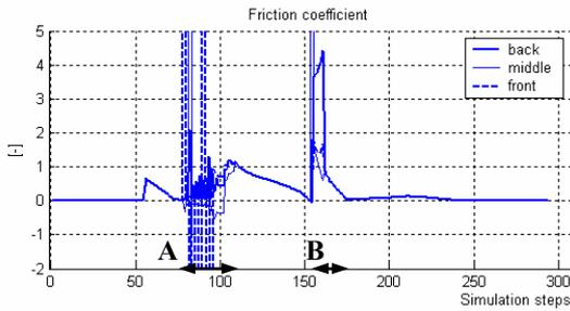
Fig. 10: Output showing the evolution of the minimum friction coefficient required. It shows clearly that the optimal solution is not found in A and B (the  $\mu$  are not equal and reach values with no real meaning).
