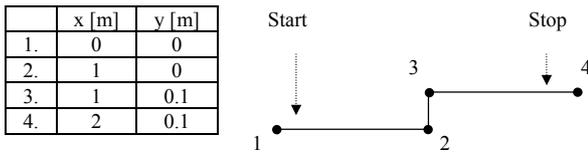
Fig. 3: Step terrain definition
