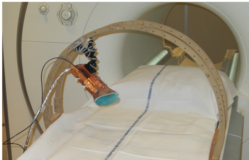
(b) The ultrasound holder is attached to the MR-compatible orbital ring using an articulated handler.
