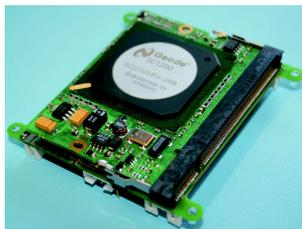
**Fig. 5.** The x-board based, 40 g and 56x71 mm computer module.
