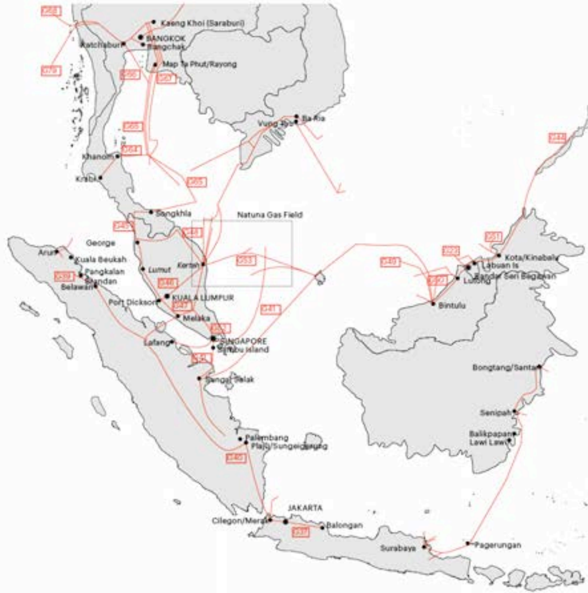
South-East Asia Pipelines Map 2011 Gas Pipeline
