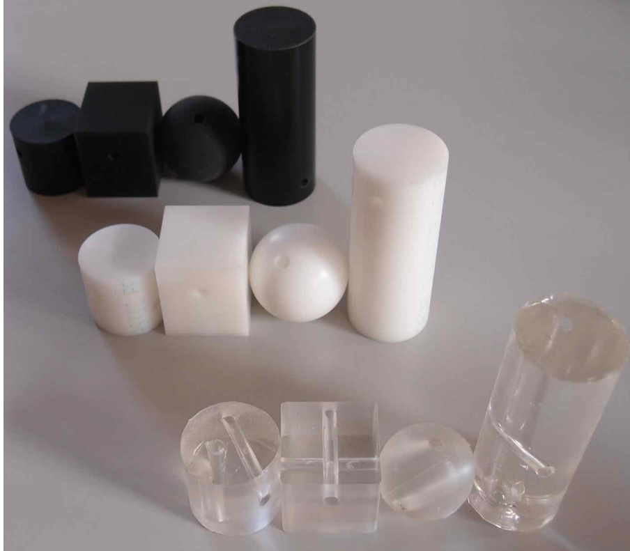
Figure 7.8: Photo of the different acoustically characterized material samples used to validate focal distortion effects induced by the presence of an inhomogeneity.
