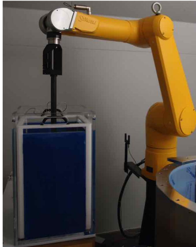
Figure 7.7: Photo of the entire measurement setup including the water-tank and the DASY52 NEO (SPEAG, Zurich, Switzerland) robot arm. The hydrophone was attached to a carbon fiber extension, which was in turn mounted to the articulated robotic arm. This setup facilitated fast and accurate measurements on a 3D grid around the geometric focus of the transducer.
