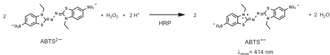
Figure 2.5.2 HRP catalyzed oxidation of \text{ABTS}^{2-} with \text{H}_2\text{O}_2 yielding the blue-green colored, stable radical \text{ABTS}^{\bullet-} .
