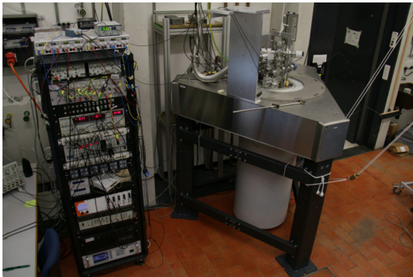
FIGURE 2.2: Photo of the 4 Kelvin MRFM system built in this work: a cryostat is on the right, and the electronics rack is on the left. The dewar is suspended by a pneumatic suspension that decouples the system from room vibrations.
