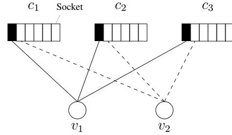
Fig. 1. A size-2 stopping set from a  $(3,6)$  random ensemble. CNs  $\{c_1, c_2, c_3\}$  and VNs  $\{v_1, v_2\}$  have been labeled for convenience. CNs have been expanded to show all their  $d_c = 6$  sockets. The solid edges indicate definite connections and the dashed edges complete one configuration to form a stopping set. Parallel edges are not allowed in the ensemble.
