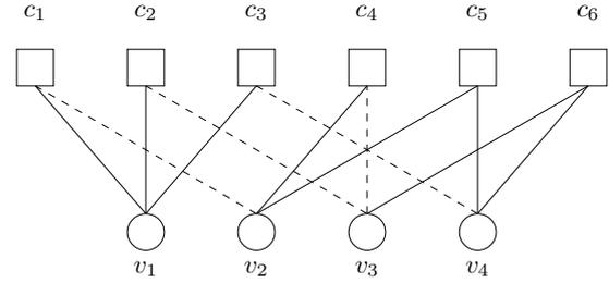
Fig. 4. A size-4 stopping set from an expurgated  $(3, 6, w, L, M)$  random ensemble. CNs  $\{c_1, c_2, c_3, c_4, c_5, c_6\}$  and VNs  $\{v_1, v_2, v_3, v_4\}$  have been labeled for convenience. The solid edges indicate definite connections and the dashed edges complete one configuration to form a stopping set. Parallel edges are not allowed in the ensemble.
