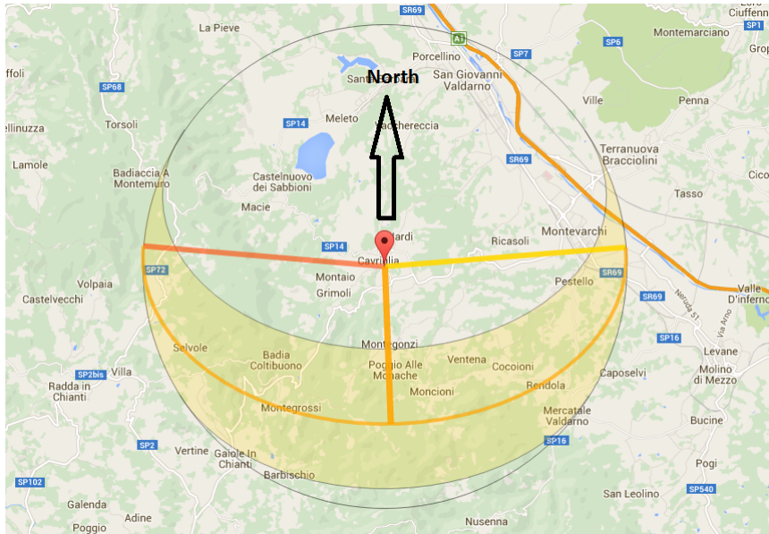
Figure 3.12: The sun path during a spring day at Cavriglia, Italy, location of ABB PV plant.
