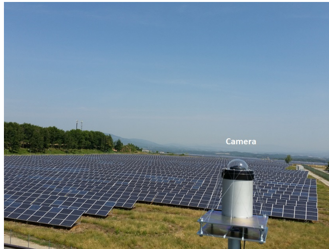
Figure 3.1: wide-angle camera system used at Carviglia site
