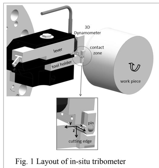
Fig. 1 Layout of in-situ tribometer
