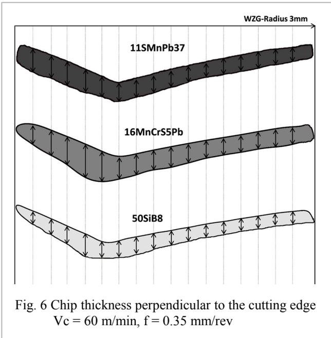
Analyzing the chip roots in X-ray tomography the whole 3-dimensional information about the chip is obtained and chip thickness (perpendicular to the cutting edge) as a function of drill tool radius-coordinates can be deduced. Fig. 6 shows a comparison between 11SMnPb37, 16MnCrS5Pb and 50SiB8 at a drilling speed of 60m/min. The machining speed then varies from zero at the centre of the hole to 60m/min at the outer radius covering the expected BUE regime.
