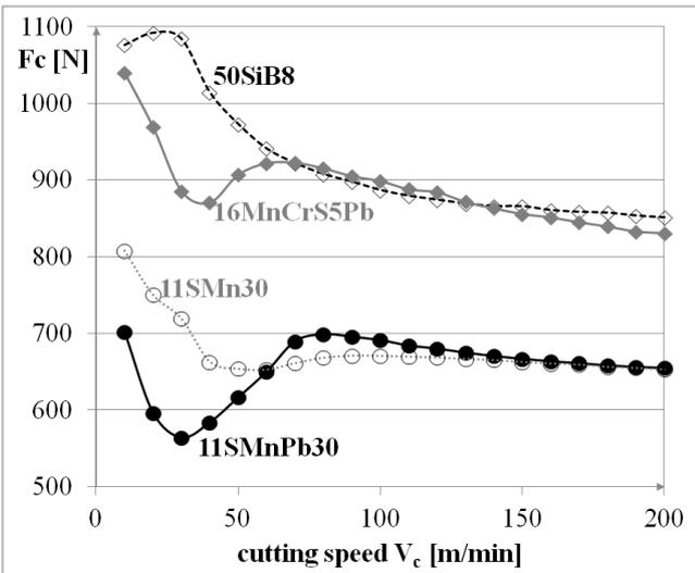
Fig. 3 Cutting forces in turning
