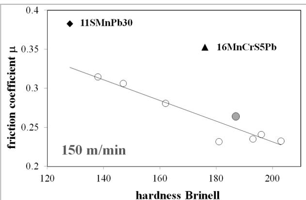
Fig. 5 Friction coefficient in dependence of hardness
