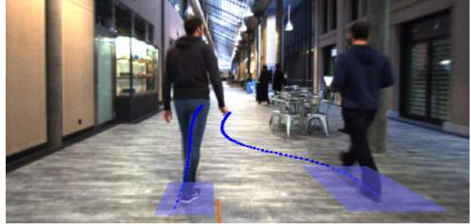
Fig. 3: Interaction features capture typical aspects of pairwise agent motion such as the agents' "private spheres". In conjunction with static obstacle information we can predict complex scenarios such as an agent (left) giving room to another due to a predicted conflict with a static obstacle.
