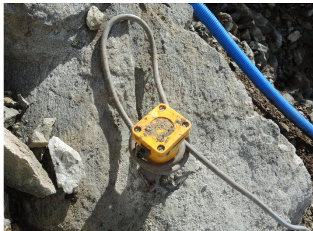
Fig. 7-3: Geophone mounted on rock as installed during the winter 2014-2015 seen from above.
