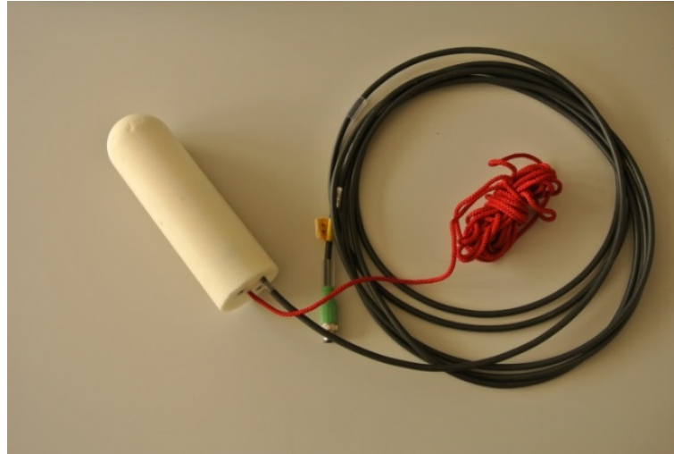
Fig. 4-2: Acceleration sensor sealed in foam cylinder (length: 20 cm, diameter: 6 cm).
