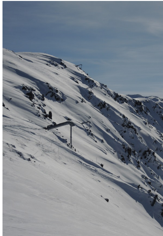
Fig. 6-1: Overview of the slope with the gas exploder. The closest gas exploder was used for the present study. The X-axis was installed on the bottom right of the gas exploder behind the lower rocks. The Y-axis was installed in the front of the picture in the slightly concave terrain. The mini-ridge probably slightly influencing the air pressure wave propagation can be seen directly at the gas exploder.
