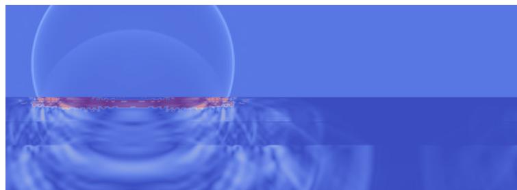
Fig. E–4: Snapshot after 2.7 ms showing the pressure in the air above the snowpack, the deviatoric (shear) stress in the subsurface (blue for positive stresses) and the locations where the maximum shear stress exceeded the strength (in red) during the time of the simulation.
