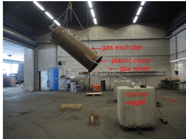
Fig. 5-1: View of the gas exploder, suspended from a crane. The pre-tensioned guy wires are connecting the gas exploder to the counterweights. The lower end of the tube is closed by a plastic cover.
