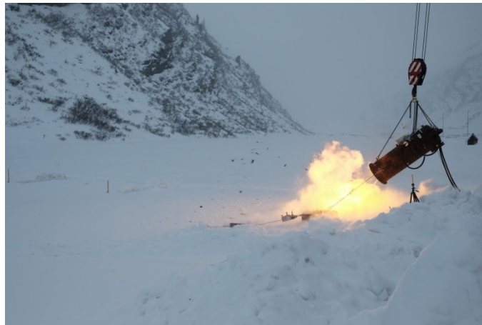
Fig. 5-3: View of the gas exploder during an experiment. Photo by M. Hiller.
