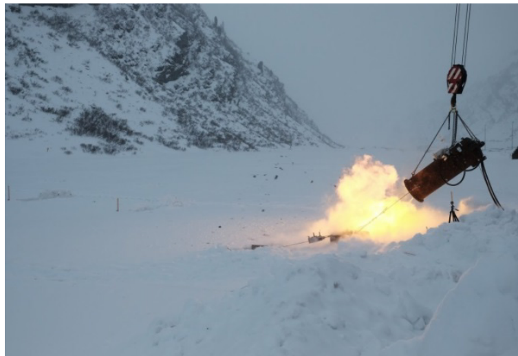
Fig. F–1: Gas exploder during explosion.
