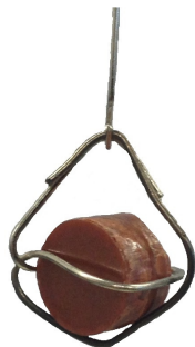
Figure 2.4. Photograph of the custom-made platinum hook suspending the dense ceria pellet to the TGA balance.
