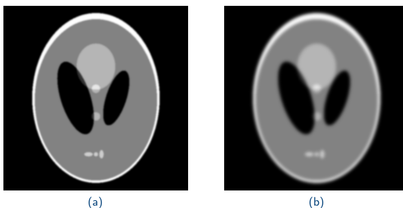
Figure 3.8: SL phantom with 512 \times 512 pixels convolved to a Gaussian kernel of radius 2 (a) and 6 (b).
