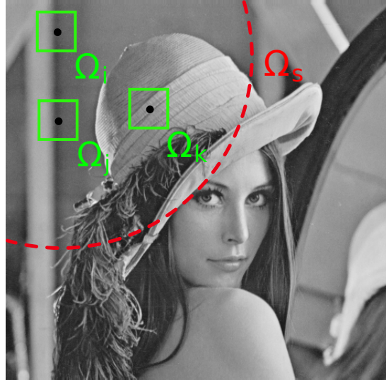
Figure 5.4: Sketch showing the mechanism of the NLM. Given a pixel i with neighborhood \Omega_i , all pixels within the window of search \Omega_s around pixel i are used to compute the similarity weights of Eq. (5.29). The weights range in [0, 1] and their value depends on the weighted square difference between \Omega_i and the neighborhood of the investigated pixel. For example, \mathbf{x}_{\Omega_j} is clearly more similar to \mathbf{x}_{\Omega_i} than \mathbf{x}_{\Omega_k} , therefore \omega_{ij} > \omega_{ik} .
