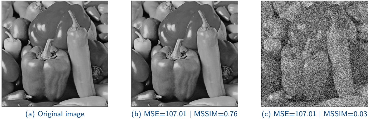
Figure 3.12: Simulation readapted from [146]. (a) Original image. (b) Image summed to a positive constant, t . (c) Image summed to t \cdot \text{rand}\{-1, 1\} . At visual inspection, the degradation of (c) is considerably more severe than that of (b). The MSE fails at identifying the difference between (b) and (c). The MSSIM, instead, succeeds.
