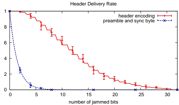
Fig. 2. Header delivery rate for our coding-based header detection algorithm and a common preamble/sync-byte-based approach. The lines show the expected theoretical results, the points the measured results; for each transmission the bit shuffling was based on a new (secret) seed. According to these results, a jammer that wants to mask a packet transmission with a probability of > 90\% would have to jam only 3 bits if the common preamble/sync-byte method is used and more than 21 bits if our coding-based detection is used. Hence, the coding-based header detection is not only much more robust than common approaches, but also facilitates the detection of a jammer as it enforces a longer jamming duration.
