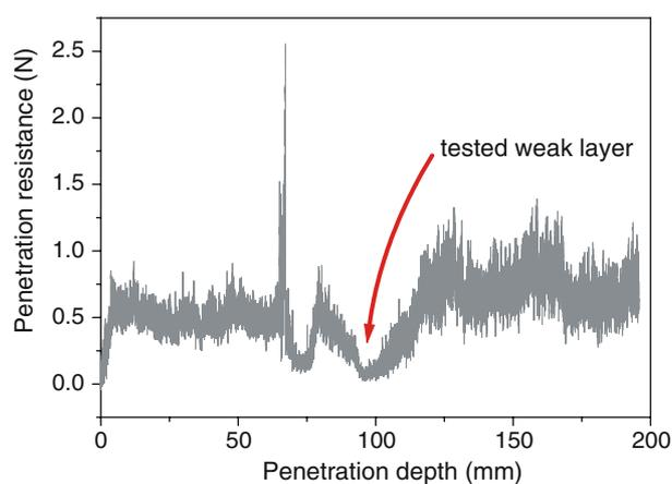
Figure 2. Penetration resistance recorded with a SnowMicroPen for Series B. The weak layer tested in series B was the layer with the lowest penetration resistance at a depth of about 100 mm.
