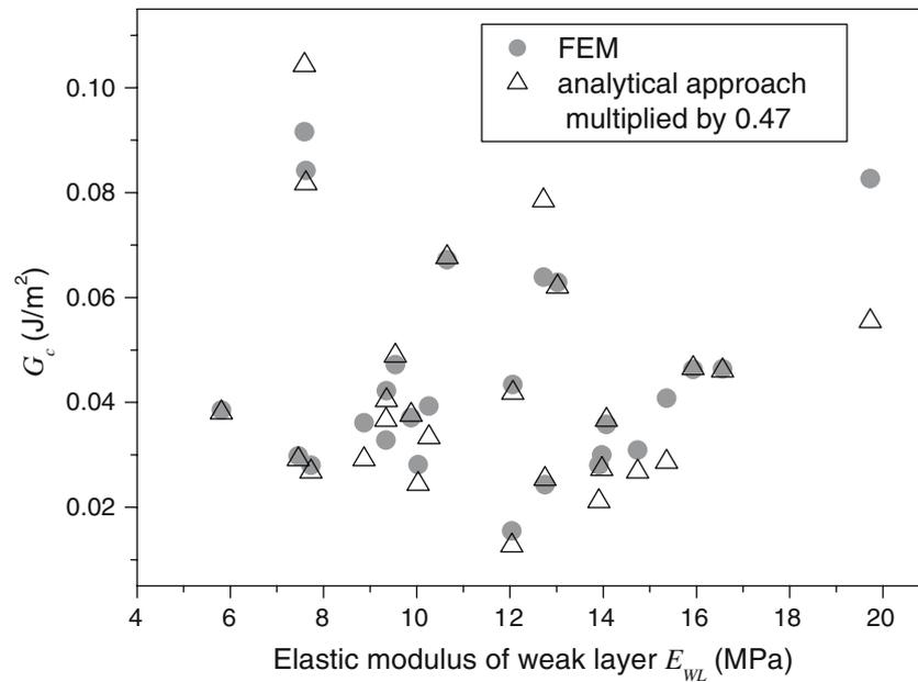
Figure 10. The numerical and analytical (cantilever beam with a deep crack) results for the energy release rate in relation to the elastic modulus of the weak layer  $E_{WL}$ . The analytical results are multiplied with a correction factor.
