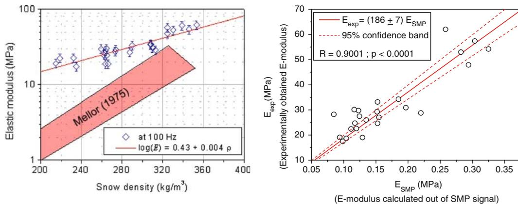
Figure 5. (a) Dynamic elastic modulus in relation to snow density, measured at a frequency of 100 Hz. Range of previous measurements summarised by Mellor (1975) are given for comparison. (b) Comparison between the dynamically measured elastic modulus  $E_{\text{exp}}$  and the modulus  $E_{\text{SMP}}$  derived from the penetration resistance signal recorded with the SnowMicroPen.
