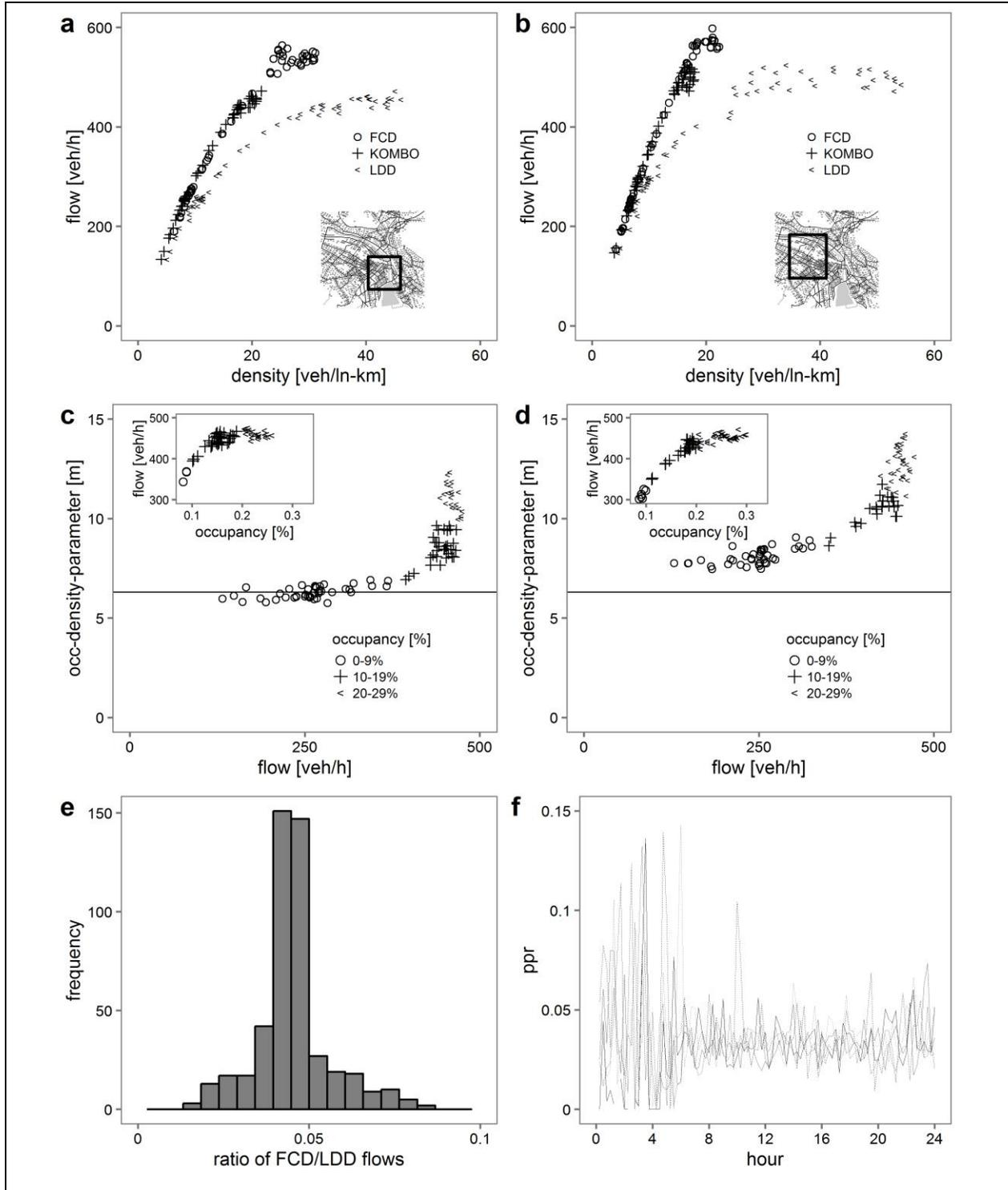
**FIGURE 3** MFD based on multiple sources. (a) MFDs for “City”, (b) MFDs for Hard, (c) occupancy-density parameter for LDD with  $x > 20$ , (d) occupancy-density parameter for LDD with projection on virtual link, (e) FCD-LDD ratio of flows, (f) estimated probe penetration rate for region “City” by time of week and day of week.
