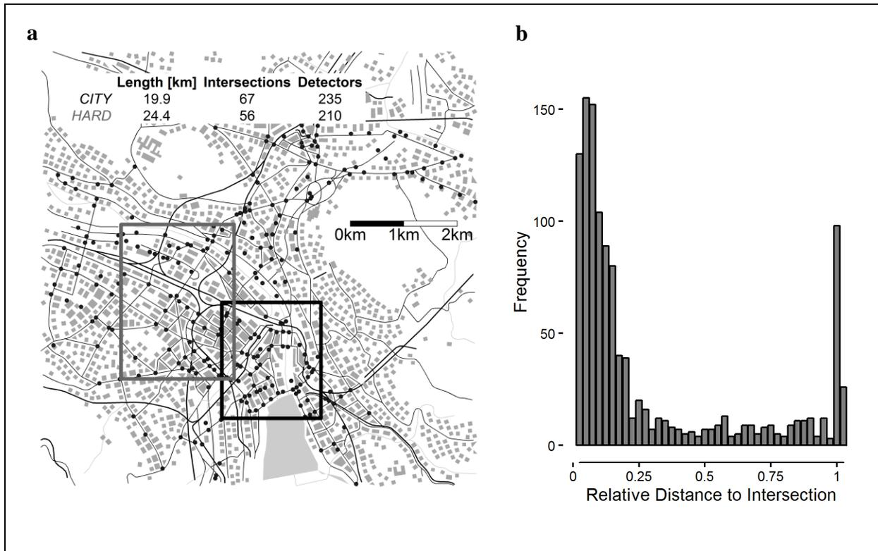
**FIGURE 1 LDD (a) Case study network, intersections equipped with loop detectors, and the two study areas used in this paper; (b) Distribution of loop detectors position on links with respect to downstream traffic signal**
