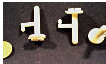
Fig. 3. “Digital” spare parts for textile machinery (Source: 3D Prints Lechthaler Reinhard)
