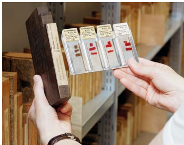
The xylotheque at the Chair of Wood-Based Materials comprises handpieces and preserved micro-specimens of wood species from all over the world, including extremely rare objects such as this ebony sample. 2014. ETH Library Zurich/Frank Blaser.
