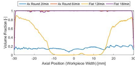
Fig. 9. Volume fraction of coolant in the grinding contact zone over workpiece width for different nozzles and flow rates.
