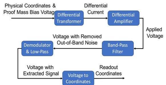
**Figure 4.** Detailed description of the sensing unit
