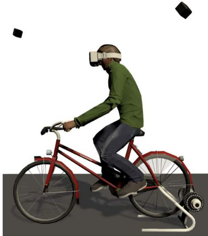
Fig. 1: Biking simulator (top to bottom): *HMD* tracking system, *HMD* as user output, bike with sensors for tracking as software input and resistance unit with bike stand.
