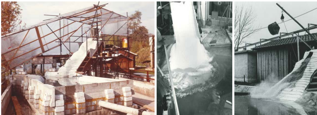
Fig. 1.5 Applied impulse wave research at VAW with scale models of prototype sites in Switzerland: Lac de Mauvoisin (VAW 1972, left), Ferden compensating reservoir (VAW 1973, center), and Lake Walen (VAW 1974, right)
