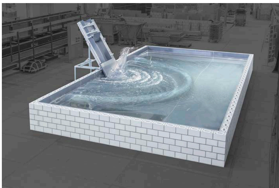
Fig. 3.6 Multi exposure picture of landslide generated impulse wave under clear-water conditions (Photo: A. Schlumpf, VAW)
