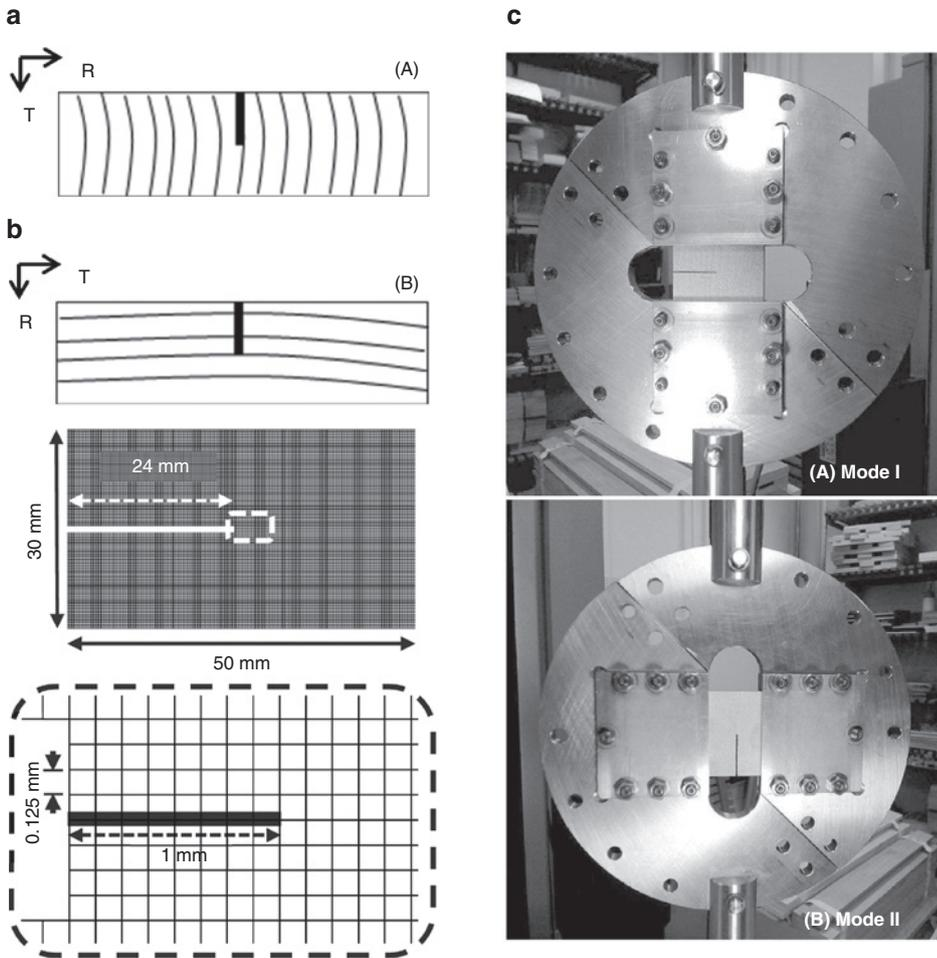
**Figure 1:** Experimental setups and a model of FEM analysis. (a) Single-edge-notch specimen. (A) RT specimen, (B) TR specimen. (b) Specimen model in the FEM analysis. (c) Set up of Arcan test attachment.
