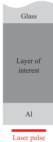
Figure 4.18: Schematic sketch of the specimens with layers from photovoltaics.
