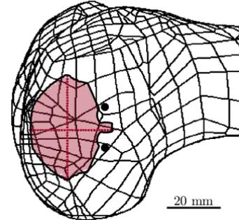
**Fig. 4** Illustration of the largest obtained planar workspace of the mechanism (in red) projected onto the femur for size relation. The anchoring points are marked by black dots. The dotted lines represent the maximal straight cuts parallel (39 mm) and orthogonal (30 mm) to the virtual line that connects the two anchor points.
