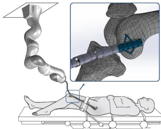
**Fig. 1** Laser osteotome consisting of a serial robot that holds a robotic endoscope ( $\varnothing$  15 mm). The end-effector (blue) of the robotic endoscope consists of a parallel robot which carries the laser optics and can be fixed to the bone which is to be cut. Figure adapted with permission from [4] and [5] (Copyright by AO Foundation, Switzerland).
