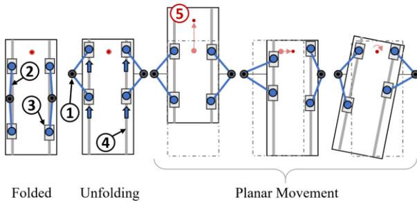
**Fig. 2** Schematic illustration of the mechanism's DoF. From left to right; Folded during insertion, unfolding and attaching by moving the four sliders accordingly, planar movement in two translations and a rotation. The mechanism's parts are: Two fixed anchoring points (1) and four legs (2) mounted on actuated sliders (3) that can move on linear rails (4) (designated by grey lines). The laser (5) operates orthogonal to the end-effector.
