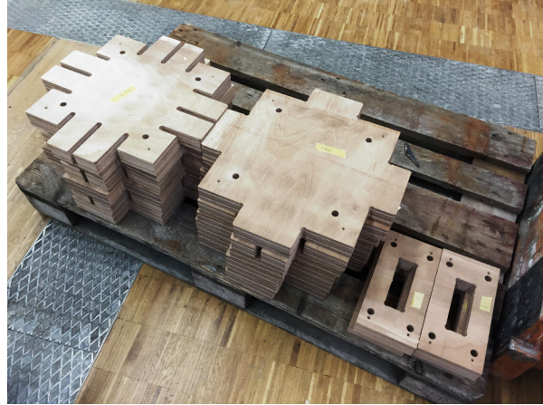
Figure 13: Specimen with different parameters, joint shapes and oversizes, 40mm thick Beech plywood.
