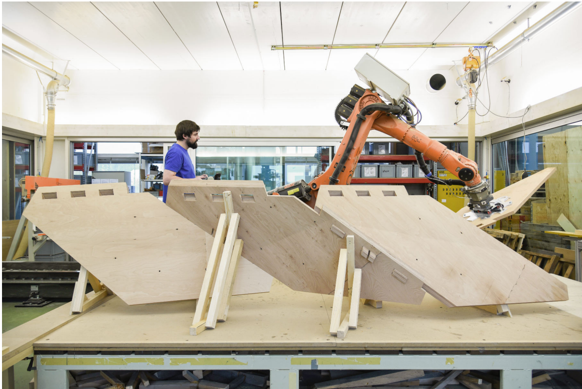
Figure 1: Large-scale robotic positioning of a timber plate.
