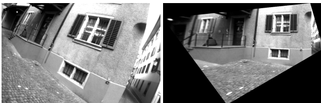
Figure 3. An example of an orthophoto (on the right) generated automatically by the proposed framework for the corresponding original image shown on the left, by estimating a local mesh illustrated in Figure 4.
