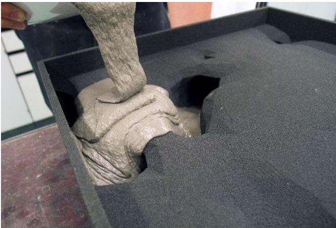
Figure 12. Casting UHPFRC inside the 3D-printed formwork.
