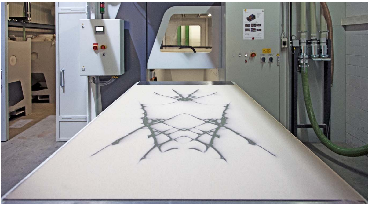
Figure 5. Industrial binder-jet 3D printer fabricating the formwork for Prototype A.
