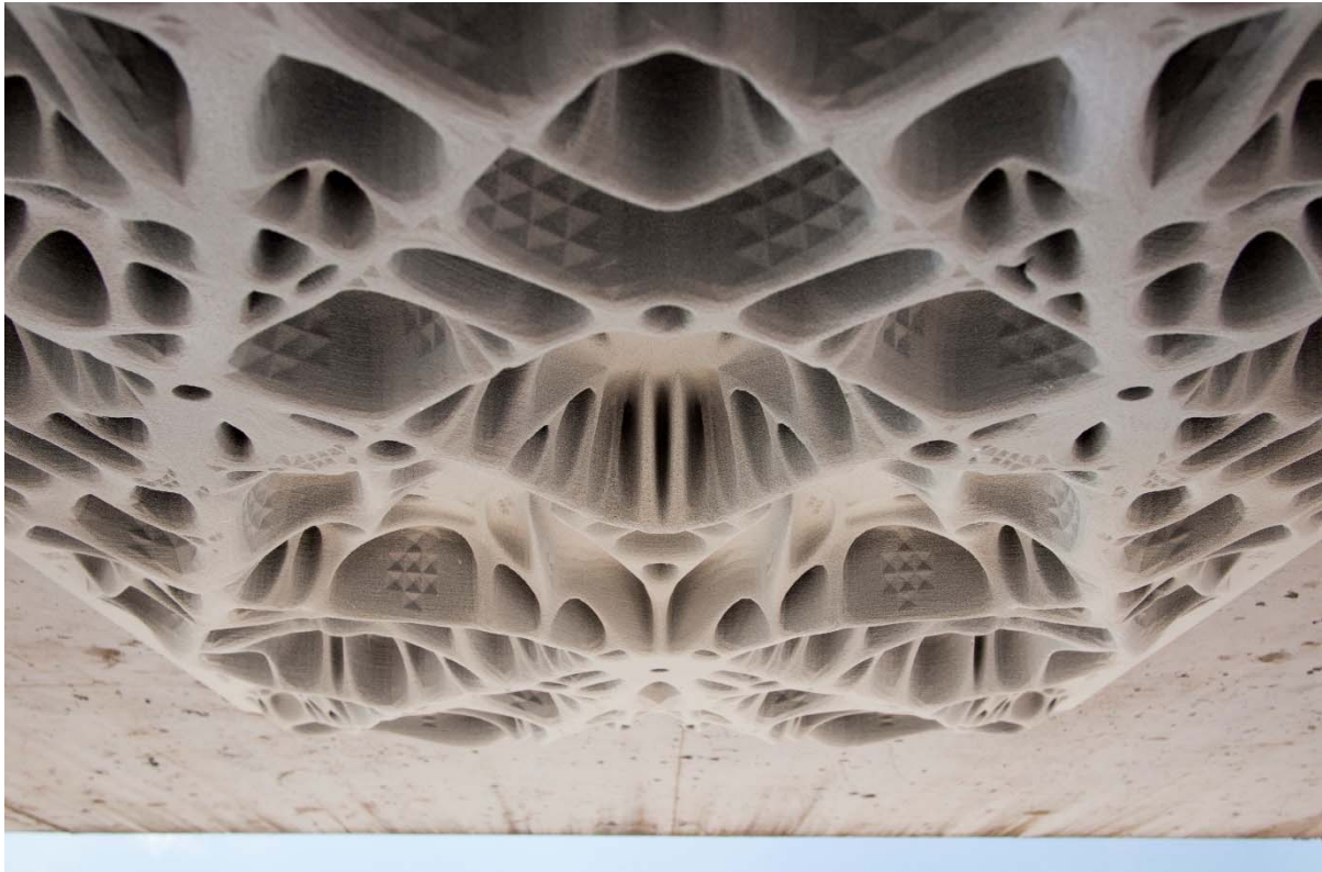
Figure 7. Detail of prototype A, showing the precise details of the finely ribbed substructure.
