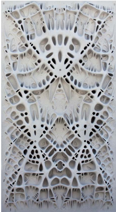
Figure 3. Prototype A: material is efficiently distributed in a ribbed substructure to reduce weight.
