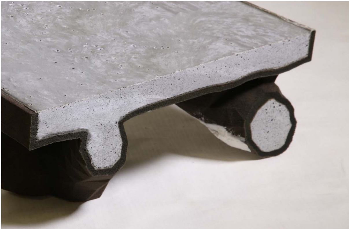
Figure 1. Stay-in-place 3D-printed sandstone formwork for high-performance fibre-reinforced concrete.
