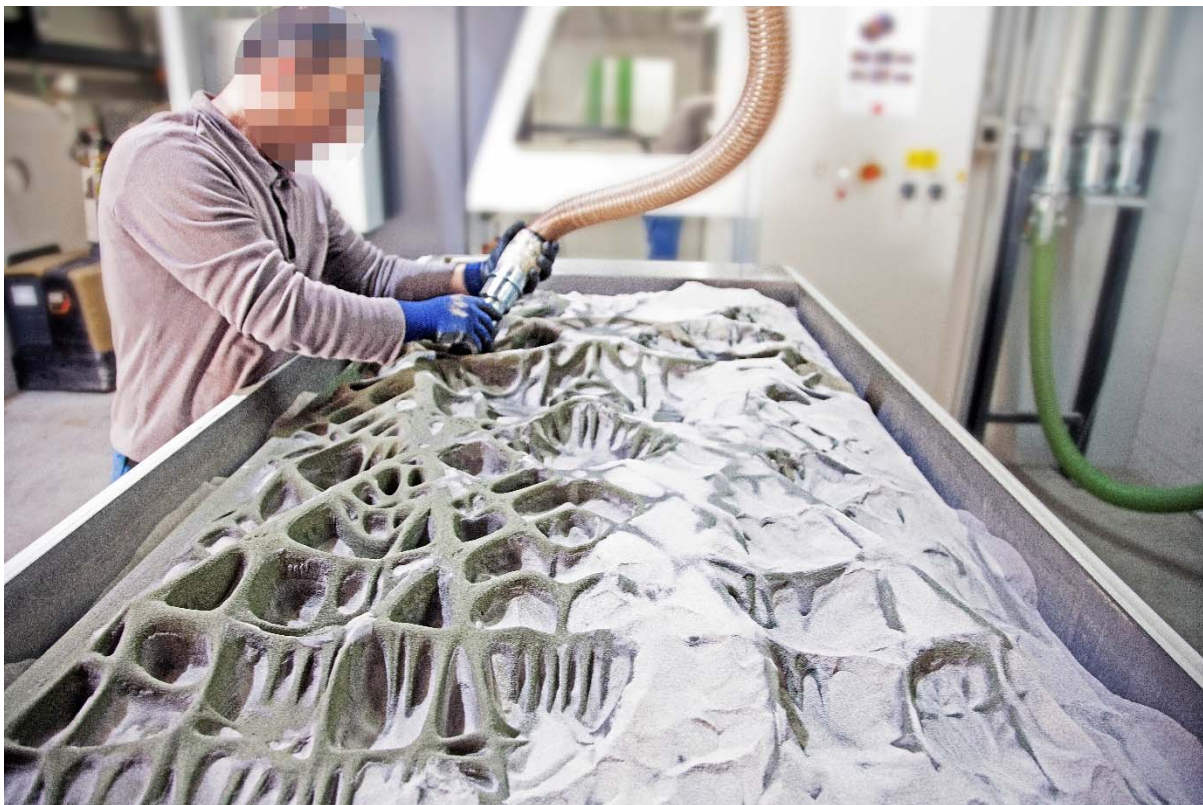
Figure 12. Post-processing of a 3D-printed sandstone formwork for prototype A.
