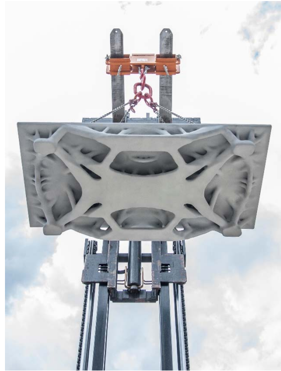
Figure 4. Prototype B: material is efficiently distributed in a porous, tubular structure to reduce weight.
