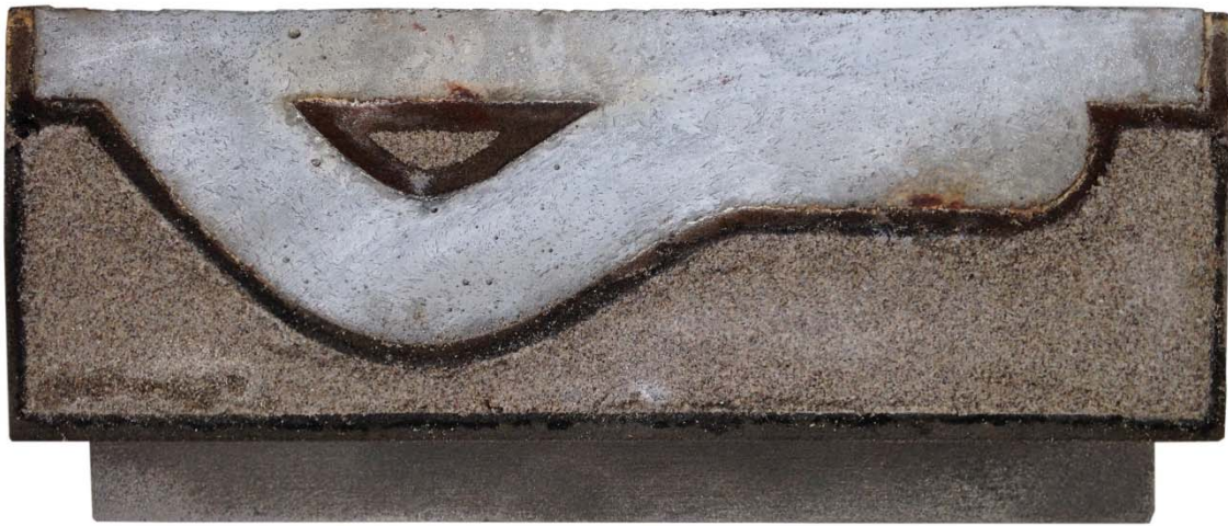
Figure 13. Integration of an auxiliary bed of unconsolidated sand contained within a closed 3D-printed box under the prototype.
