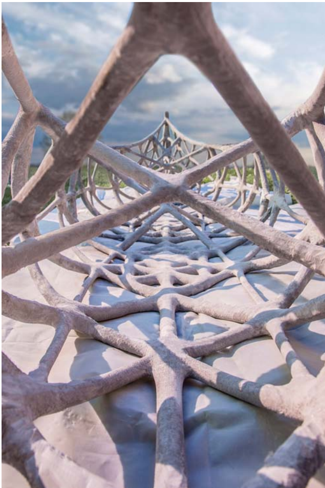
Figure 2: The complex concrete “skeleton” which provides the structural integrity for the canoe (DBT, ETH Zürich, 2017)
