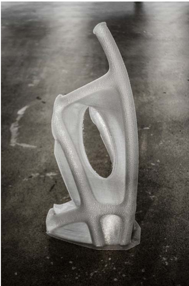
Figure 7: A 700mm tall sample 3D printed part of the SkelETHon formwork. In order to prevent quality issues for taller parts, a membrane-like auxiliary support structure is introduced. (DBT, ETH Zürich, 2017)
