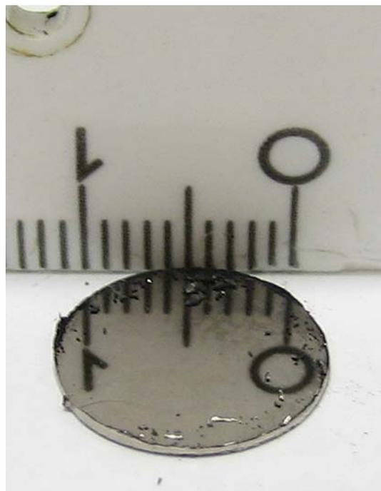
Figure 5. Bulk pill pressed from bismuth nanopowder pressed uniaxially at 370 MPa. The nanocrystalline metal is highly reflecting as can be seen from the mirror image of the white ruler (cm scale).
