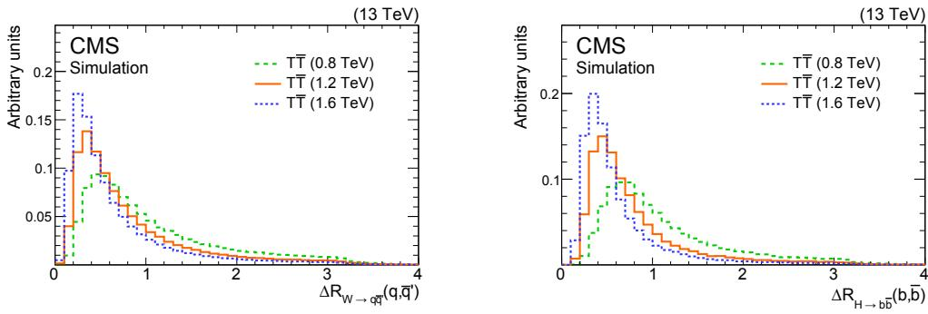
Figure 2. Angular separations  $\Delta R$  between the products of simulated  $W \rightarrow qq^0$  (left) and  $H \rightarrow b\bar{b}$  (right) decay processes for three different mass points of the  $T$  quark. Even for the lowest mass point shown, the final state particles are typically emitted with a separation of  $\Delta R < 0.8$  and are merged into an AK8 jet.
