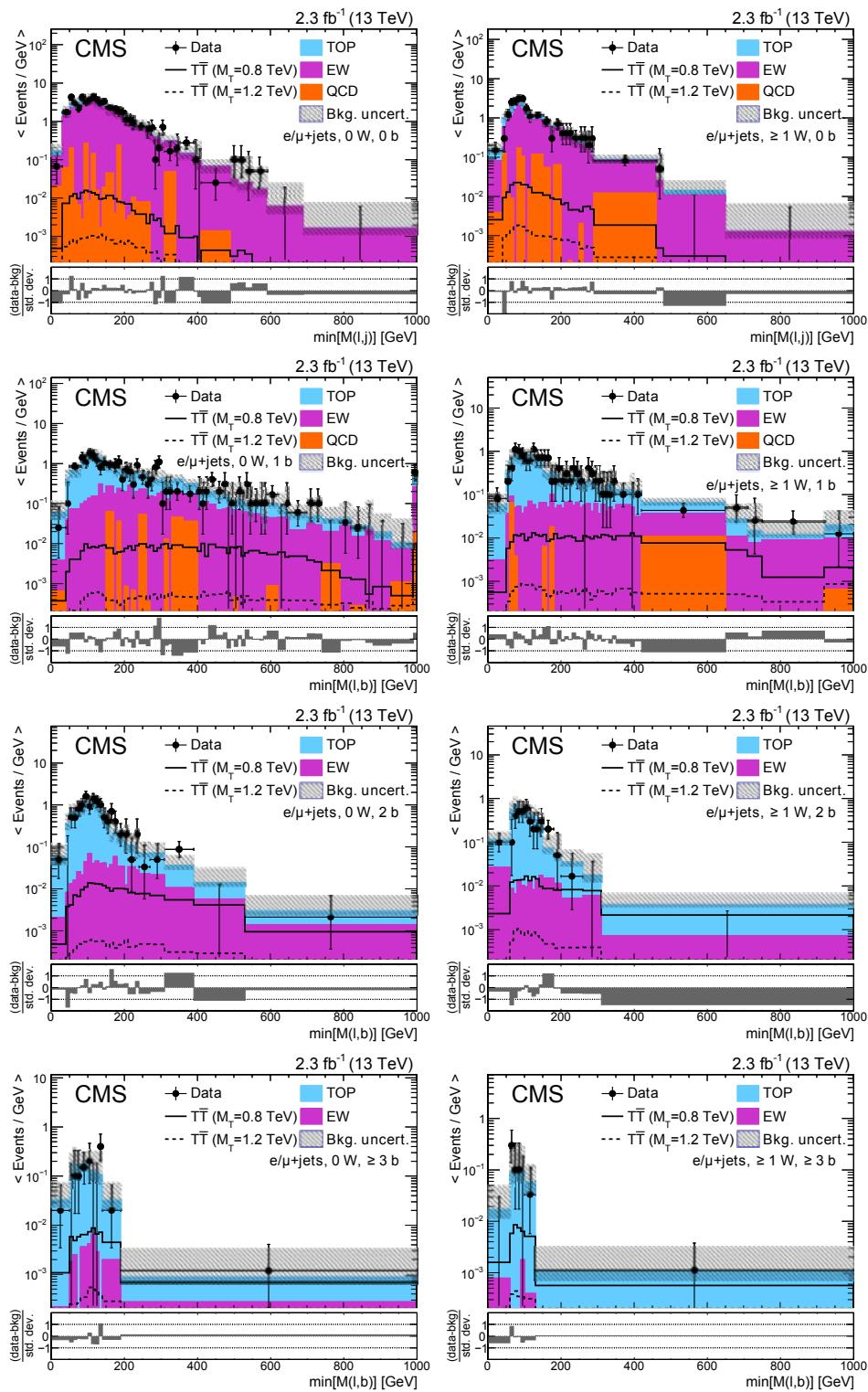
**Figure 9.** Distributions of  $\min[M(\cdot; j)]$  or  $\min[M(\cdot; b)]$  in the combination of electron and muon channels in the boosted  $W$  categories with 0 (left) or (right)  $W$ -tagged jets and (upper to lower) 0, 1, 2, or  $b$ -tagged jets. Also shown are the distributions of  $T\bar{T}$  signal events with  $T$  quark masses of 0.8 and 1.2 TeV. The uncertainty in the background includes the statistical and systematic uncertainties described in section 7.
