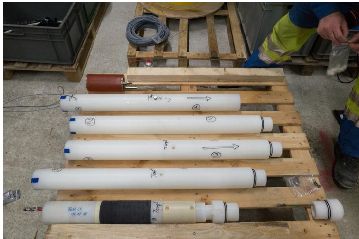
Figure B-13: SBH 15.004 packer system
