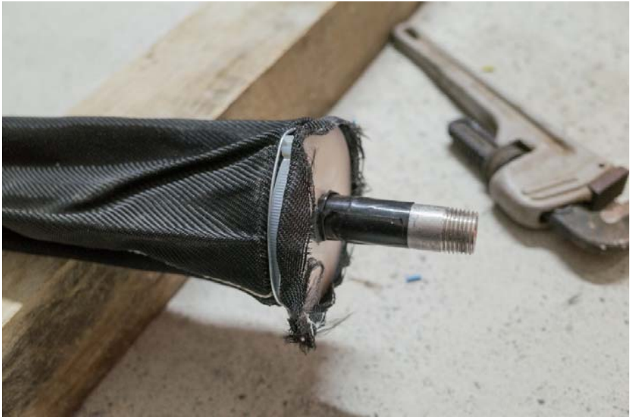
Fig. 2. Preparation of the bottom packer with the geotextile sleeve mounted to the bottom disk.
