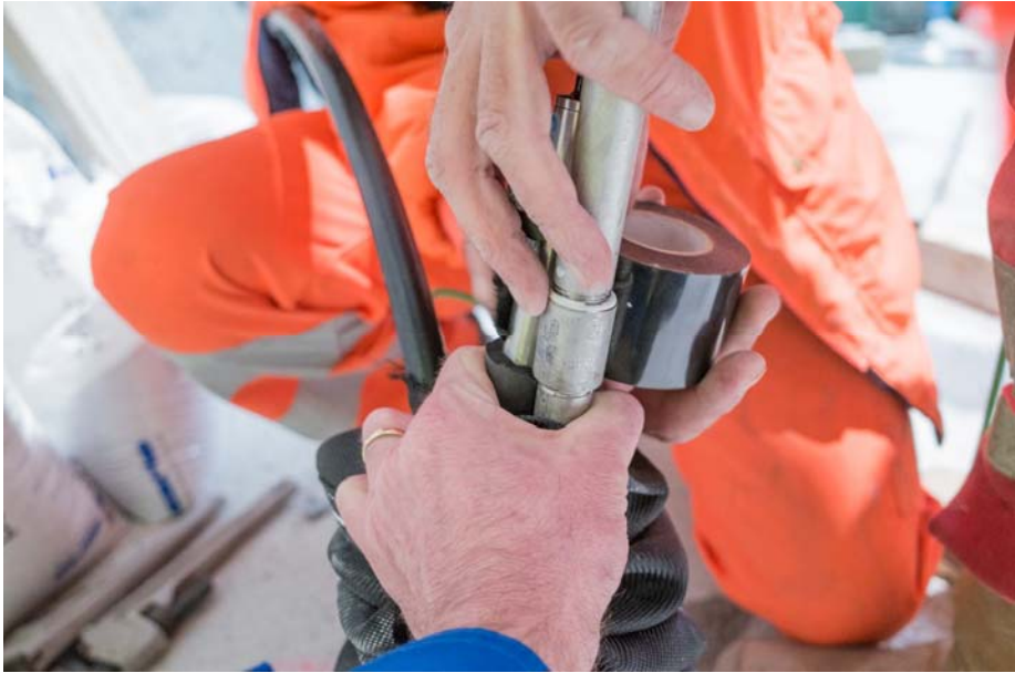
Fig. 3. Attaching a pressure sensor to a fitting of the central tube with adhesive tape."
