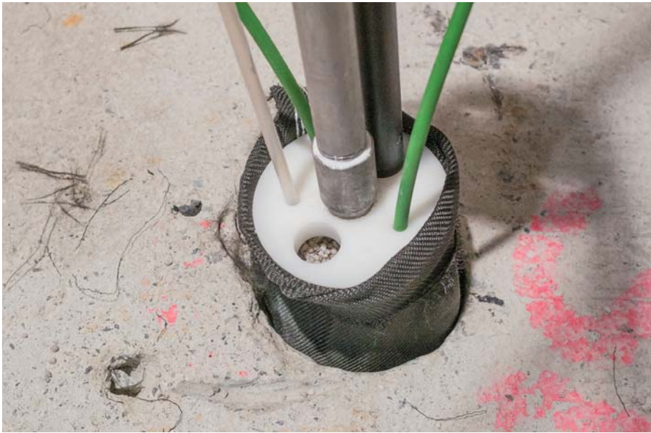
Fig. 5. Central interval section completely filled with quartz sand.
