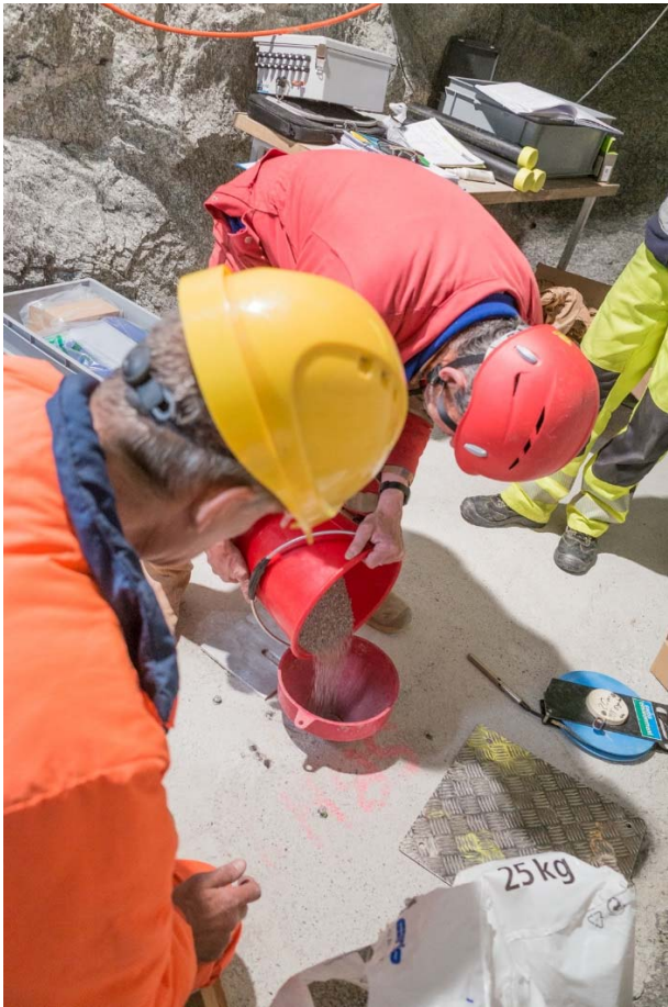
Fig. 1. Filling the bottom interval section with quartz sand.
