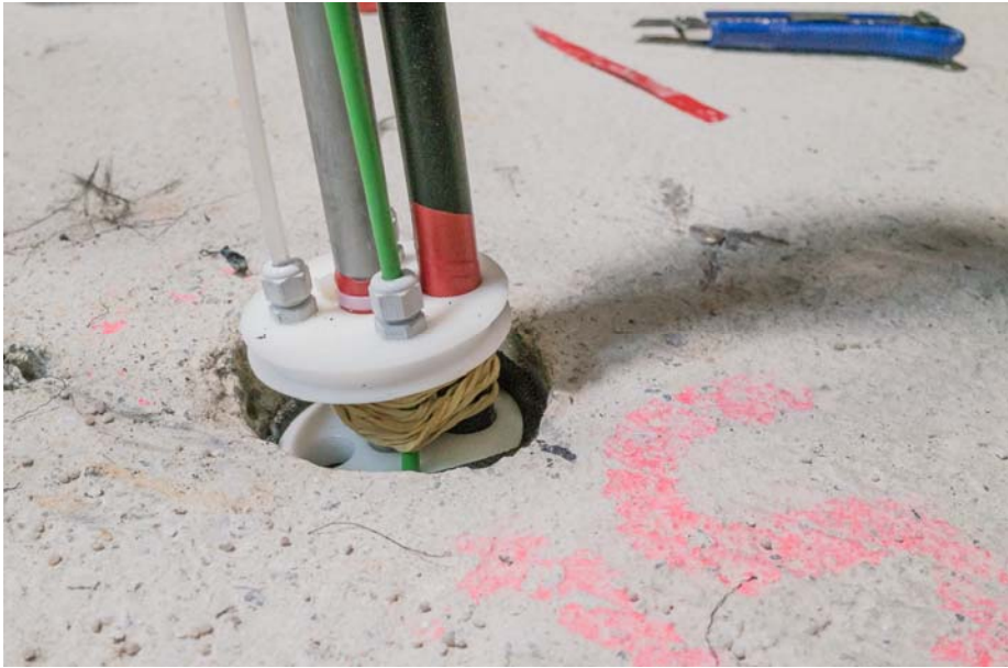
Fig. 6. Top disk of lower interval section and bottom disk of central grout-packer.
