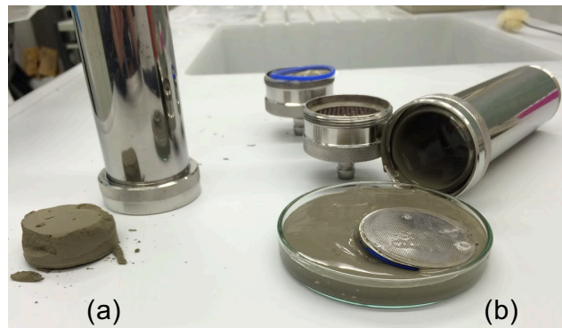
Figure I.1: Effect of the filtration for 10 minutes under pressure of 50 g (a) and 150 g (b) of a cement paste prepared with 4 mg/g active by weight of cement of 2.5PMA1000 at w/c ratio of 0.3.
