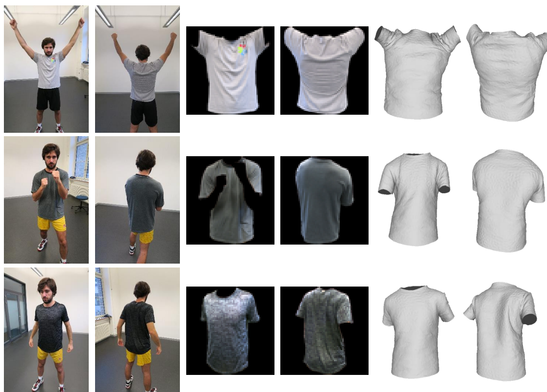
Figure 4.13: Estimated garment shapes from two views. From left to right: original image from the front and back, image after segmentation (input image) from the front and back, view of the estimated meshes from the front and back.
