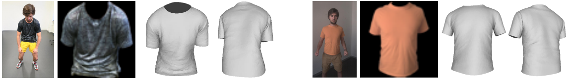
Figure 4.1: Garment 3D shape estimation using our CNN model and a single-view. From left to right: real-life images capturing a person wearing a T-shirt, segmented and cut-out garments and 3D estimations of the shape.
