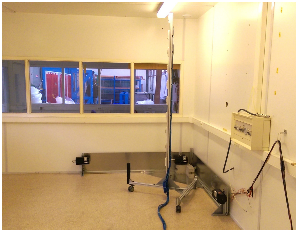
Figure 44: The small-scale prototype of the magnetic field mapper. The mobile tower houses ten fluxgate magnetometers. A bundle of readout cables is visible at the bottom of the tower. Behind it a rigid L-piece is visible, which holds three string potentiometers. A wire is extended from each potentiometer to the tower.
