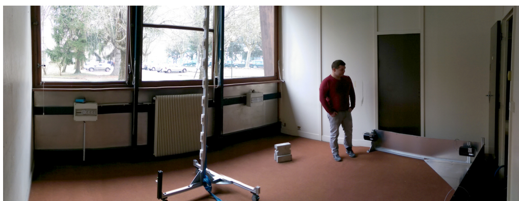
Figure 76: A photograph of the “chalet” room at LPSC Grenoble. On the picture visible are: the “L-piece” holding string potentiometers (to the right), the mapping tower with magnetic field sensors, a large steel radiator (below the window).
