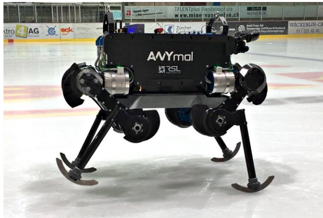
Fig. 1. The robot ANYmal [2], [3] performing skating motions on ice.
