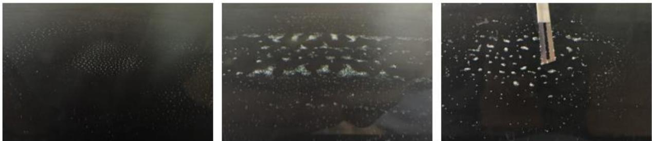
**Fig. 10. The pattern of bubbles on the test surface at the location of the ultrasonic transducer**
