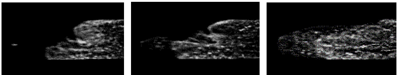
29.37500 ms 29.44375 29.54375 Fig. 6. High-speed video observation at DDT in 11.4% C 2 H 2 + 28.6% O 2 + 60% N 2 at 13.6 kPa
