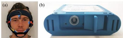
Figure 1 (a) Frontal biosignal recording with fixation headband and integrated headphones. (b) Mobile acoustic stimulation device.
