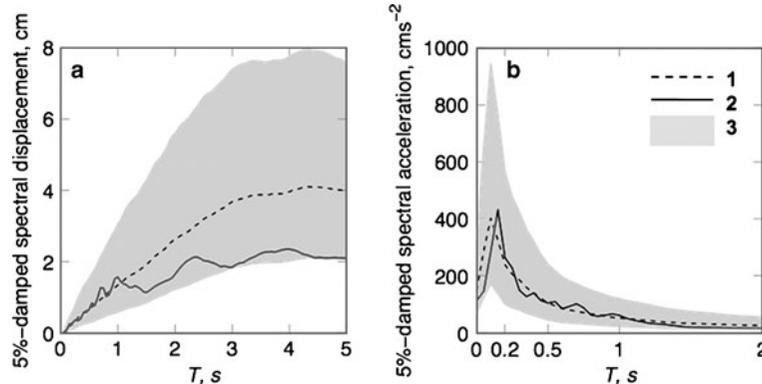
**Fig. 9** Elastic 5% damped spectral displacements (a) and pseudo-accelerations (b) at Tarcento for the Sept. 15, 1976 (09:21)  $M_W$  6.1 Friuli aftershock. Hypocentral distance from TSH is equal to 19 km. Curves 1 represent the median response spectrum prediction by Cauzzi and Faccioli
