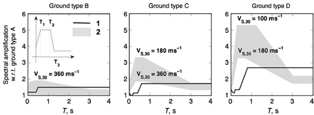
**Fig. 13** Spectral envelopes (shaded bands 2) of site amplification, as given by Eq. 1 for ground type *B*, *C*, and *D*. 1 is the spectral amplification due to site effects as prescribed by the Eurocode 8 (CEN 2004)
